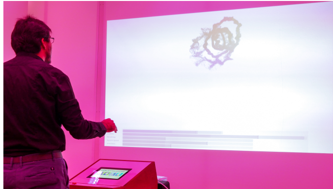
Figure 1. Con Espressione! Exhibit at the “La La Lab – The Mathematics of Music” exhibition. The hand movements are tracked with a LeapMotion sensor, enabling the user to shape overall tempo and loudness of the performance. The Basis Mixer (BM) adds more subtle performance characteristics, such as micro timing. The contribution of the BM can be controlled and experimented via a slider. The higher the value, the more freedom does the BM have in adding deviations from the prescribed parameters.
